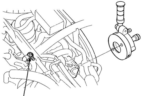
6. Tighten the adjusting screw lock nut and recheck the flow rates. Adjust as necessary.
