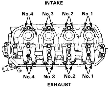
2. Set No. 1 piston at TDC. "UP" mark on the pulley should be at top, and TDC grooves on the pulley should align with cylinder head surface. The distributor rotor must be pointing towards No. 1 plug wire.
