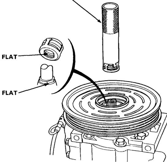
15. Clean the seal seat with cleaning solvent, then lubricate the seal seat with refrigerant oil (SUNISO 5GS or equivalent).
