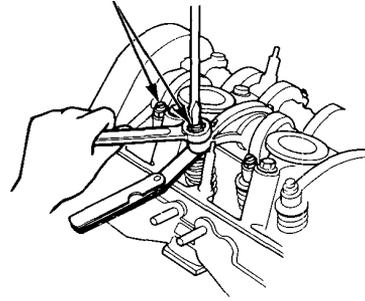
5. Tighten locknut and check clearance again. Repeat adjustment if necessary.
