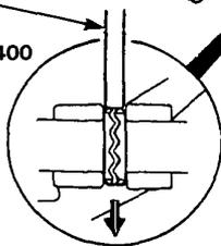
**CAUTION:** Do not lose the spring-loaded detent while disassembling the shift forks and shift fork shafts.
