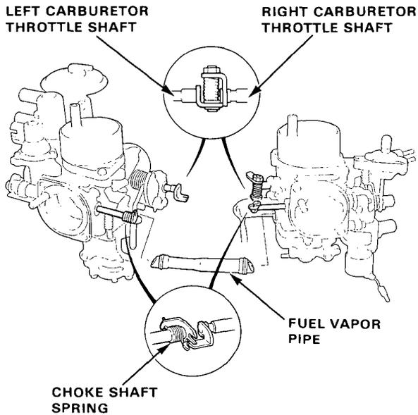
4. Connect the choke shaft spring.
