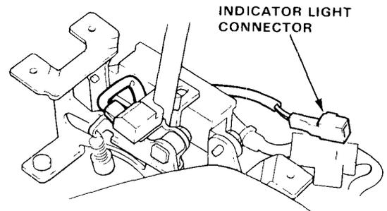
2. Install the indicator bulb in the bulb housing. Insert the bulb housing into slot in escutcheon, then turn 90° to bulb housing.
