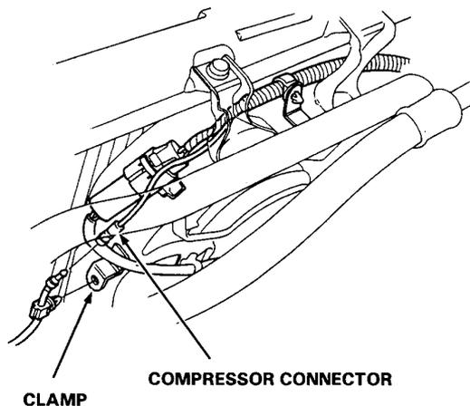
6. Loosen the adjusting bolt and lock nut, then remove the compressor belt.
