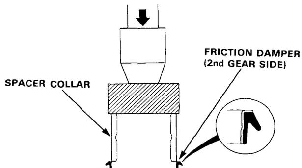
3. Install the ball bearing using a press as shown.
