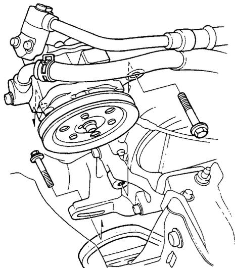
4. Disconnect the suction and discharge hoses from the compressor.
