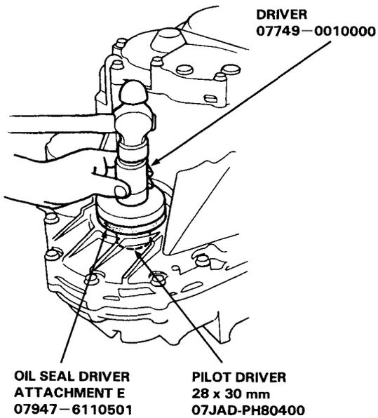
2. Install the oil seal in the torque converter housing.
